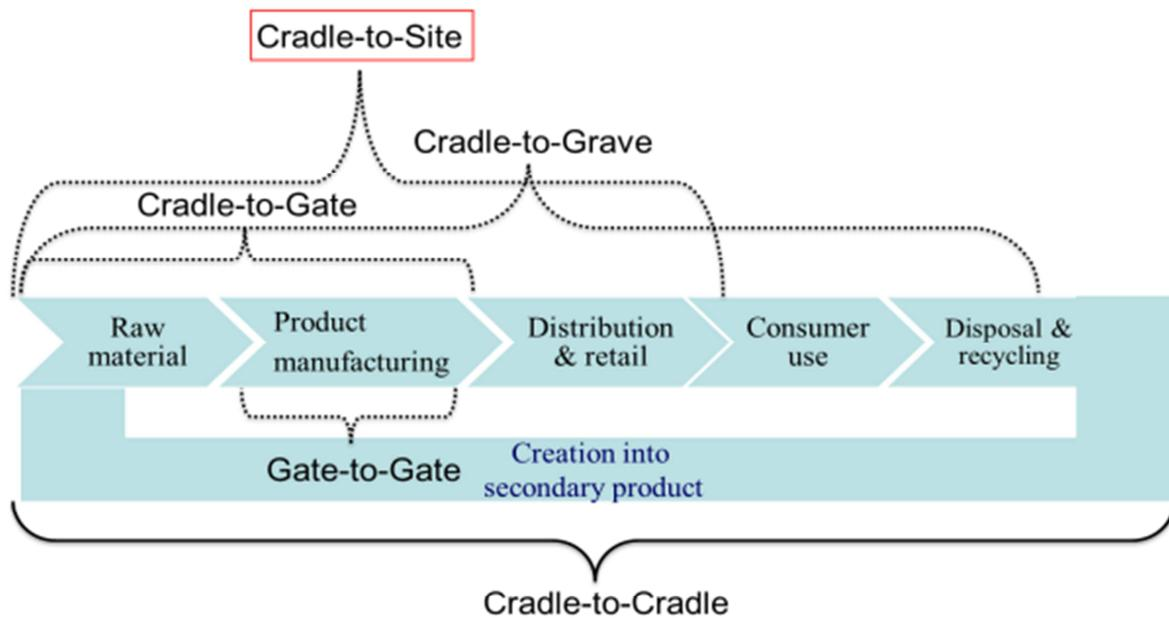
**Figure 4 System Boundary of Life Cycle** (Jack C.P. Cheng et al.)
