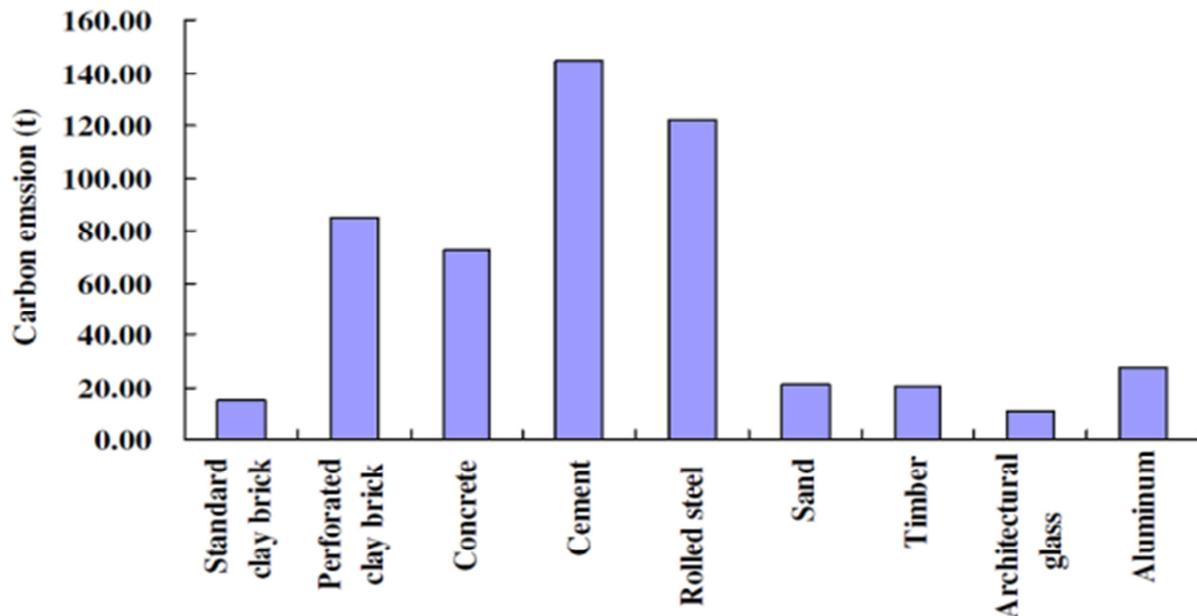
**Figure 7 The Carbon Emission of Main Construction Materials in Nanjing, China (Nick Lewis)**
