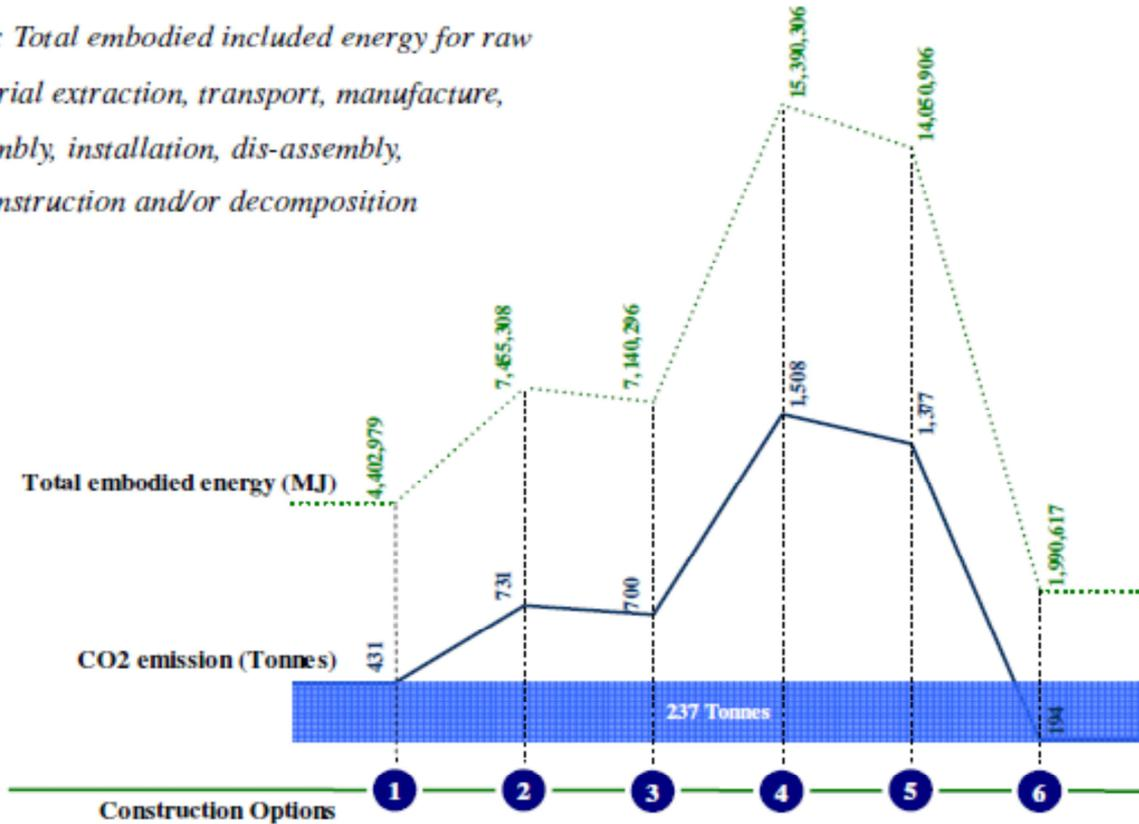
**Figure 8 Resulting embodied energy and possible CO<sub>2</sub> emission (kg CO<sub>2</sub> ≈10.204 MJ) for different construction options (Gary S K Chou)**
