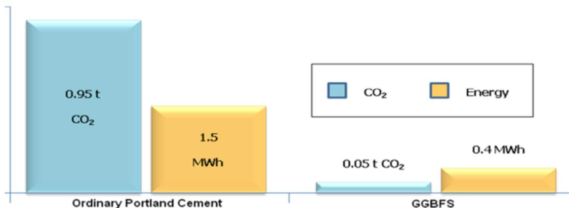
Figure 9 Comparison of energy and embedded CO<sub>2</sub> per ton of OPC & GGBFS (Nick Lewis)
